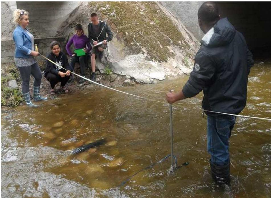
Fig. 2 – Field measurement of flow velocity
