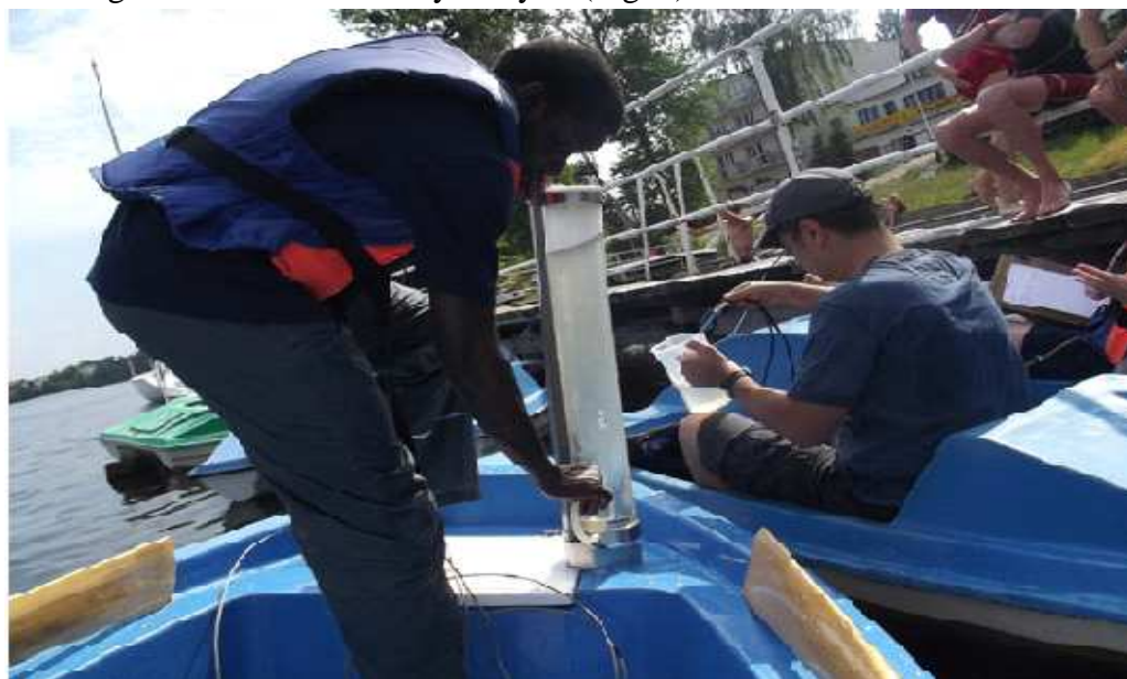
Fig. 6: Water sampler being used to collect water samples at various depths for chlorophyll a measurement
