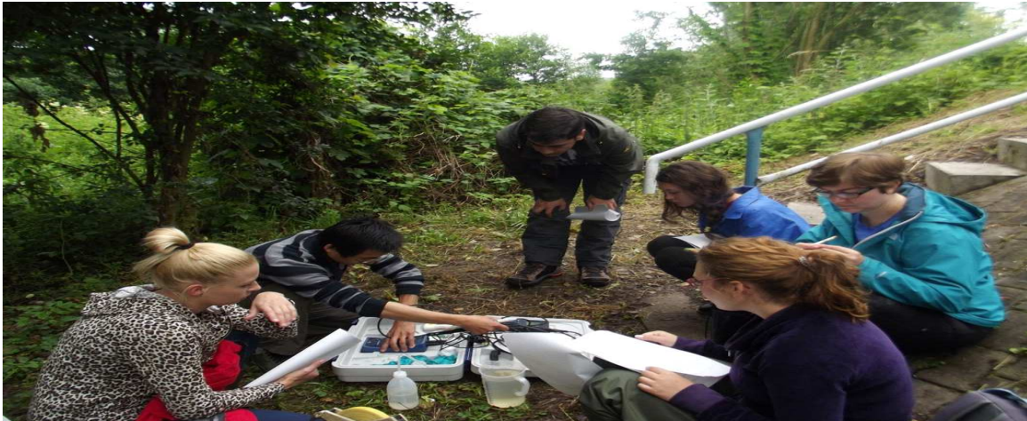
Fig. 7 pH, Electrical conductivity, Oxygen concentration, Temperature measurements with WTW Multi Parameter Meters
