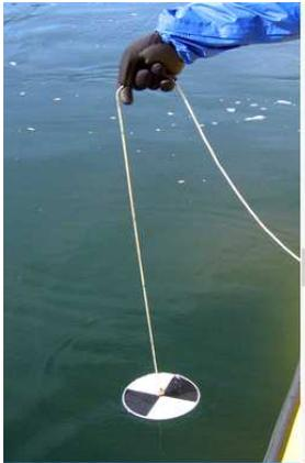
Fig. 5: Turbidity measurement with Secchi disk (SD)
