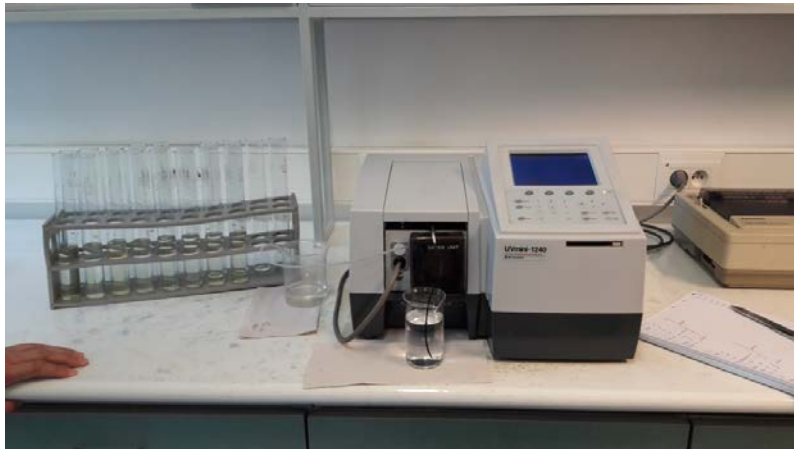
Figure 3. Photometer used for nutrient measurements.
