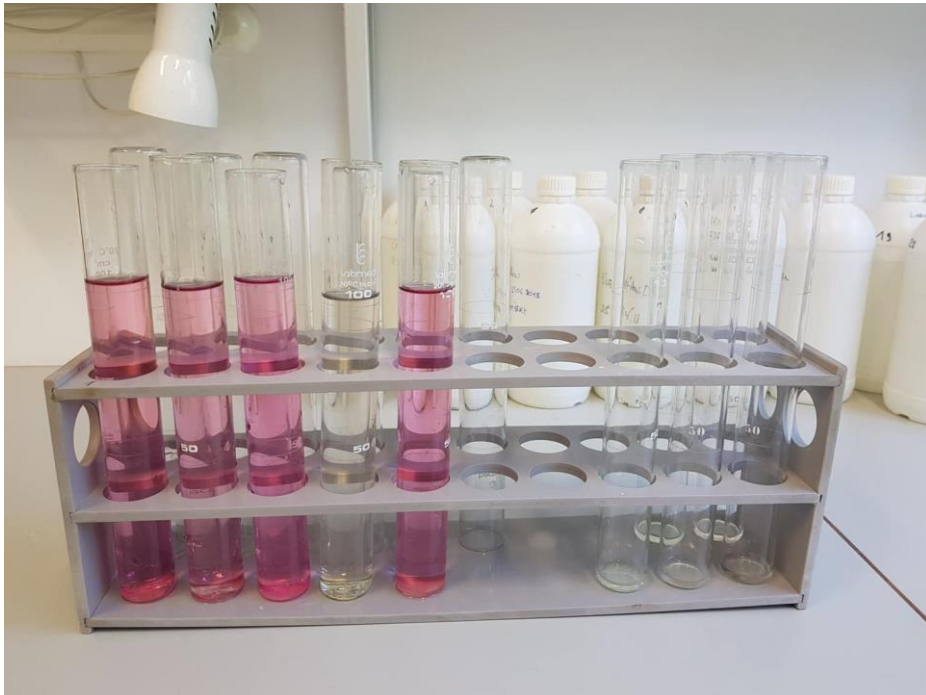
Figure 10. Properly prepared samples showing different amounts of nitrite nitrogen inside
