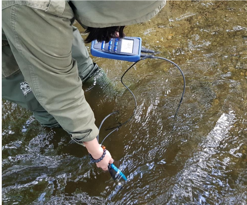
Figure 4. The measurement of pH, dissolved oxygen and temperature in situ
