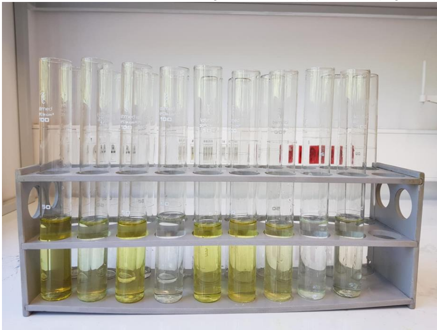
Figure 9. Properly prepared samples showing different levels of ammonium nitrogen concentration.
