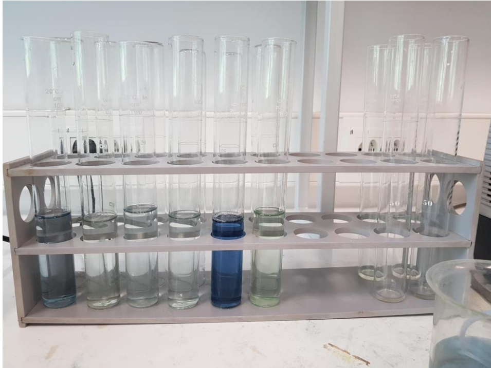
Figure 11. Properly prepared samples, showing different amounts of phosphate concentration
