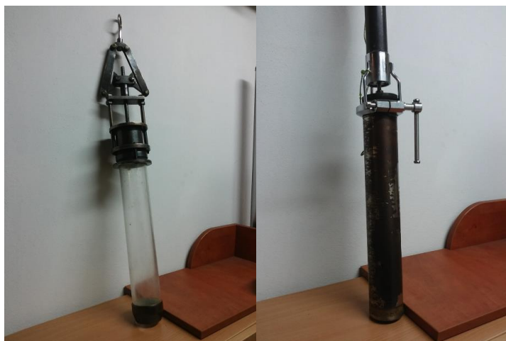
Figure 3 – Pictures of the two core samplers used for the collection of samples of macroinvertebrates: (a) Kajak corer (b) Czaplą corer
